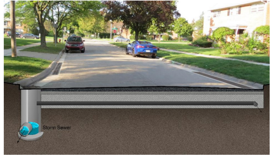
Trench drain to stone reservoir across full street
