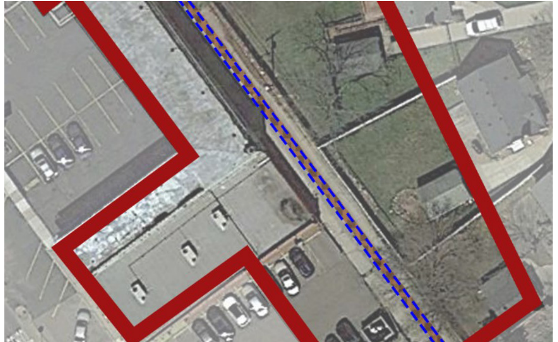
3 ft Wide Center Strip of Permeable Pavers, Full Length of Alley or Catch Basins (not shown)
